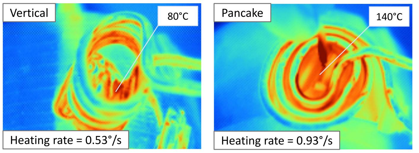
Figure 3 – Thermal imaging of a vertical and a pancake coil.
