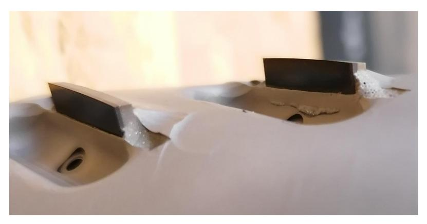
Figure 2 – Aluminium milling tool prototype after EDM sharpening.
