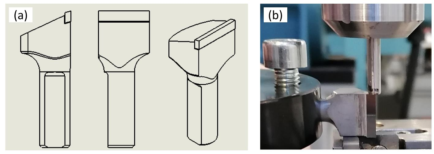
Figure 1 – Real joint specimen geometry (a) and shear testing setup (b).
